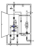
CAB Megatron® with SS cabinet around mixing valve
